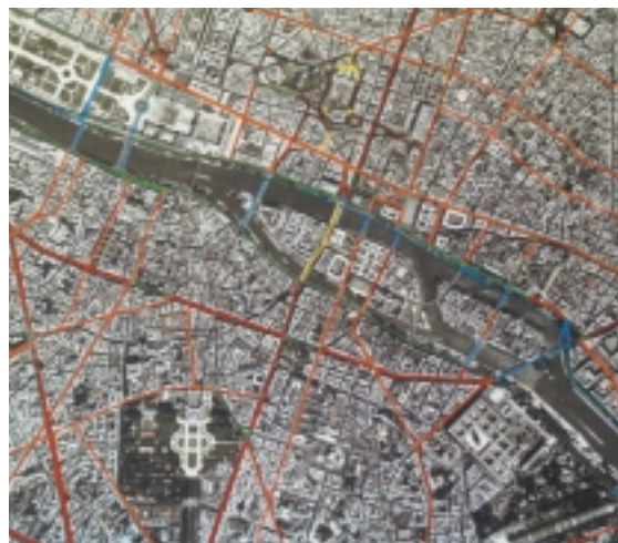
Figure 4: Description of the road typology - Example of Paris City Centre. Each colour is associated to a reference road typology (i.e. canyon street, large avenue)
